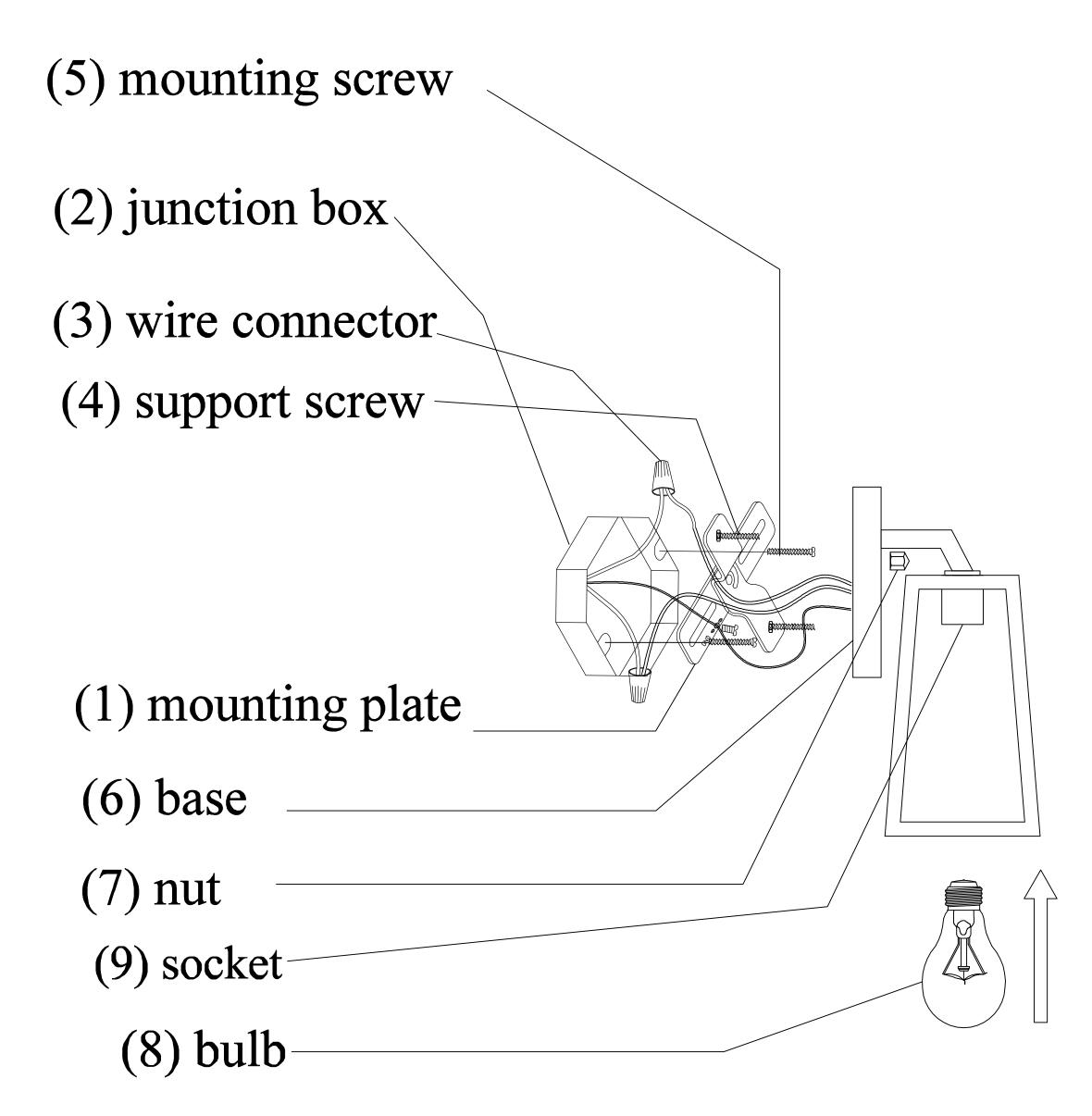
Please turn off power to the outlet and review instructions before installation. The installation must be handled by a qualified licensed electrician. Also, be sure to turn off power before changing the bulb or cleaning the fixture.
