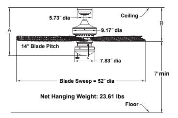
Ceiling fan attaches to electrical junction box securely anchored and capable of withstanding a load of at least 50 lbs.
